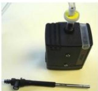
1. Use Tubelock tool to remove both brass end caps.
